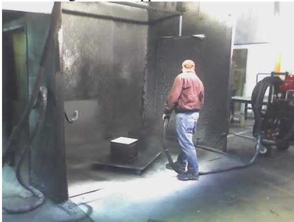
A typical O.E.M. Polyurea application spray booth.
